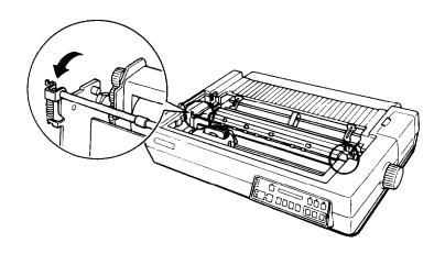
4. Hold the assembled cut sheet feeder in both hands and fit its notches over the red pins in the printer.
